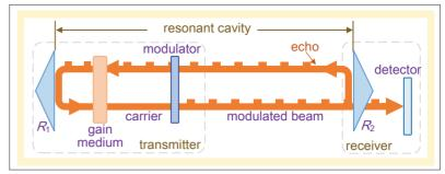
Figure 5. Echo interference in a resonant beam communications system.
