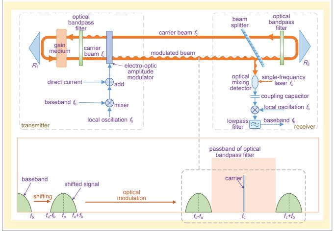
Figure 6. Exemplary design with echo interference elimination.
