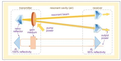
Figure 2. Resonant beam system mechanism.
