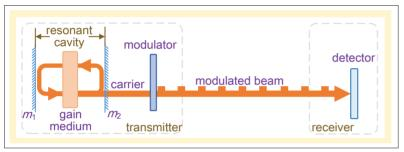
Figure 4. Laser communication system.
